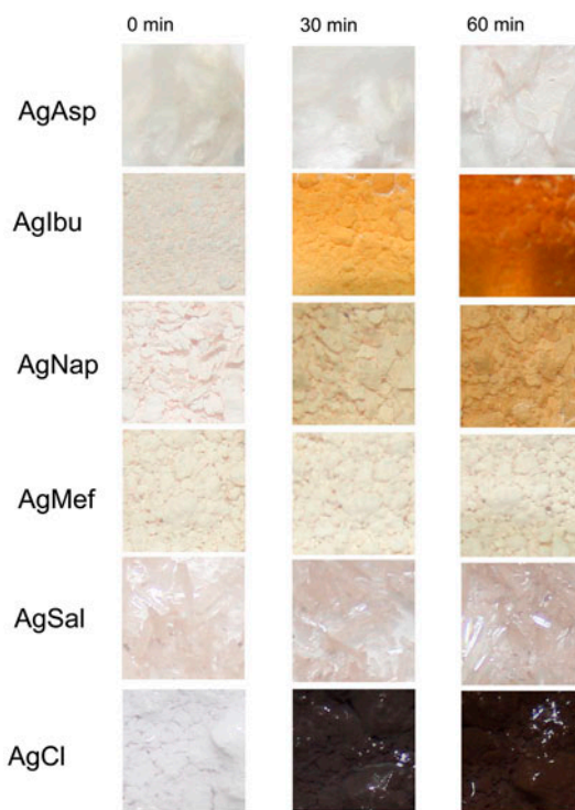
Figure 10. Reduction of synthesized silver(I) compounds in presence of high-energy UV radiation at 258 nm and 30 watts. Five water soluble silver(I) complex with Ibuprofen (AgIbu), Naproxen (AgNap), Mefenamic acid (AgMef), acetyl salicylic acid (AgAsp), and salicylic acid (AgSal). From Azocar et al. [61].
